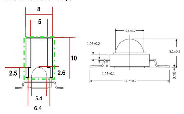
(the inner diameter of the nozzle the untouchable moliding colloidal)
