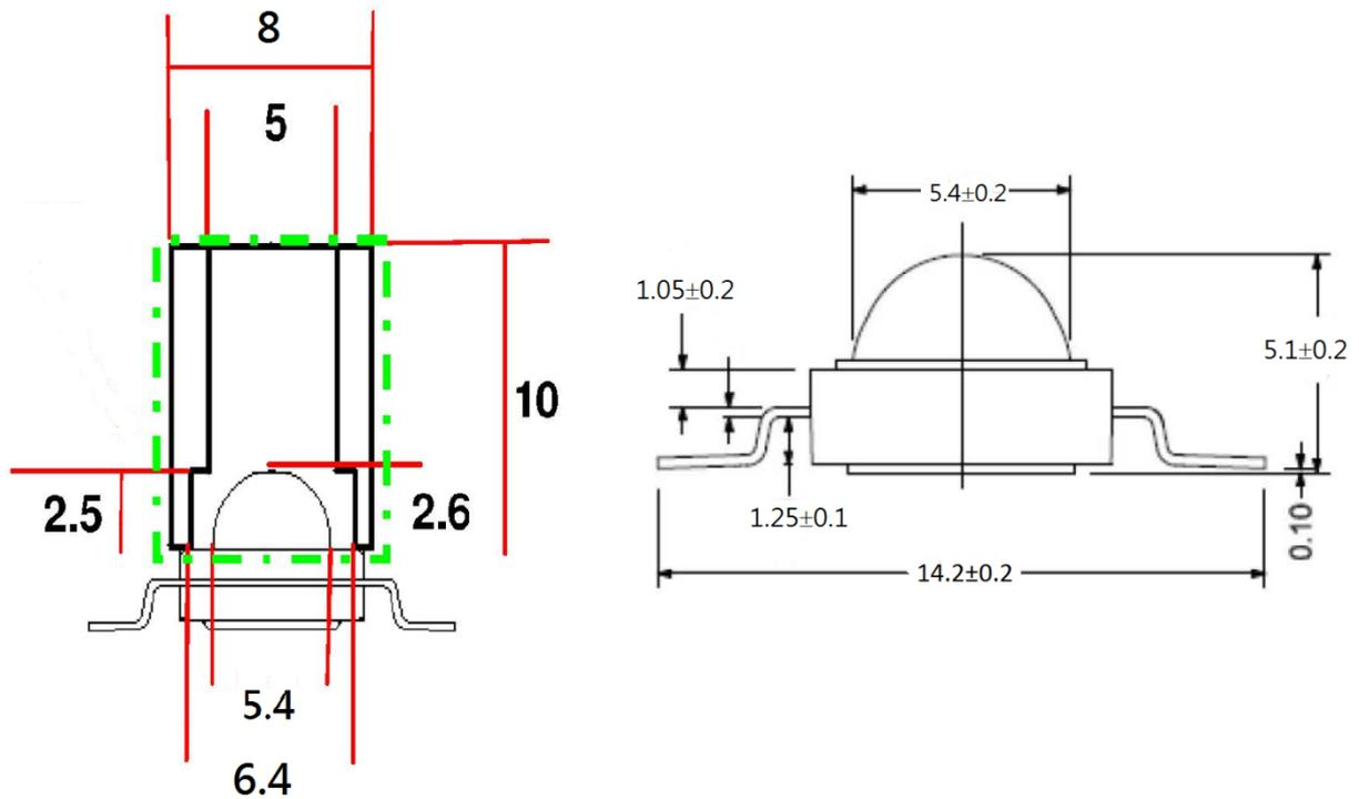
(the inner diameter of the nozzle the untouchable molding colloidal)
