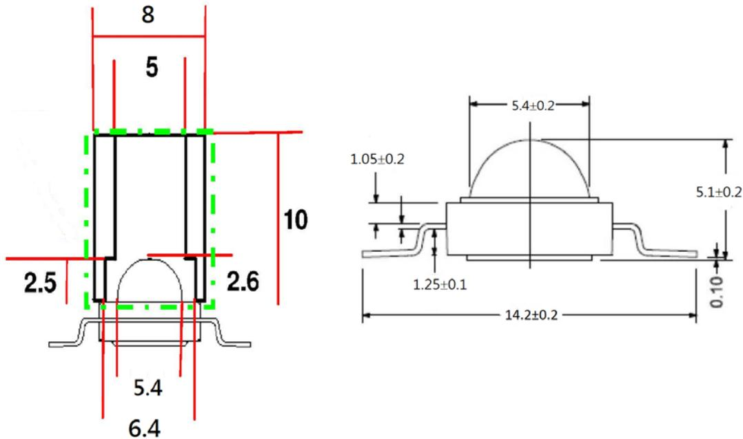
(the inner diameter of the nozzle the untouchable molding colloidal)
